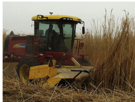
Fig. 1. A self-propelled mower-conditioner (New Holland model H8080: 750 HD specialty rotary disc head, New Holland, PA) used in mowing miscanthus.
