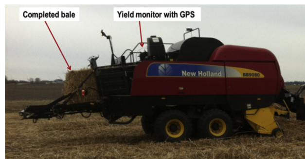
Fig. 2. Large square baler (New Holland model BB9080, New Holland, PA) used in harvesting experiments.
