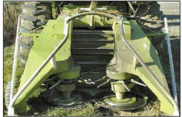
Fig. 1. Particular of the GBE-1 header for SRF harvesting.
