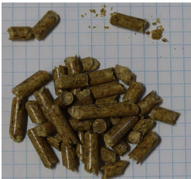
Fig. 1 – Modern cylindrical biomass pellets. Top-left: usual mode of fracture. Top-right: fines produced by scraping a fingernail across the end of the pellet. Bottom: bulk pellets. Grid paper is 6.35 mm for scale.
