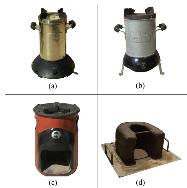
Fig. 1 – Photographs of the cookstoves tested. (a) Philips forced draft (PF), (b) Philips natural draft (PN), (c) Envirofit front feed (EN), (d) Traditional brick-mud cookstove (TR).
