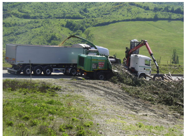
Fig. 1 – Truck-mounted independent-engine chipper (Unit 1).
