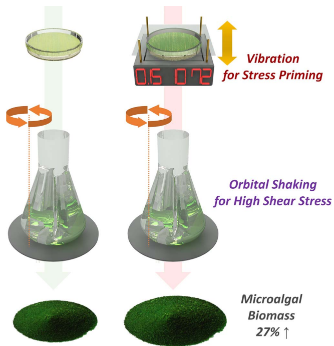
Fig. 1. Schematic representation of the two steps for microalgal stress priming: the vibration generation system for stress priming (top right) and the baffled flask shaking incubator for high shear stress (middle). These steps were compared with the steps from a seed plate (top left) as a control.
