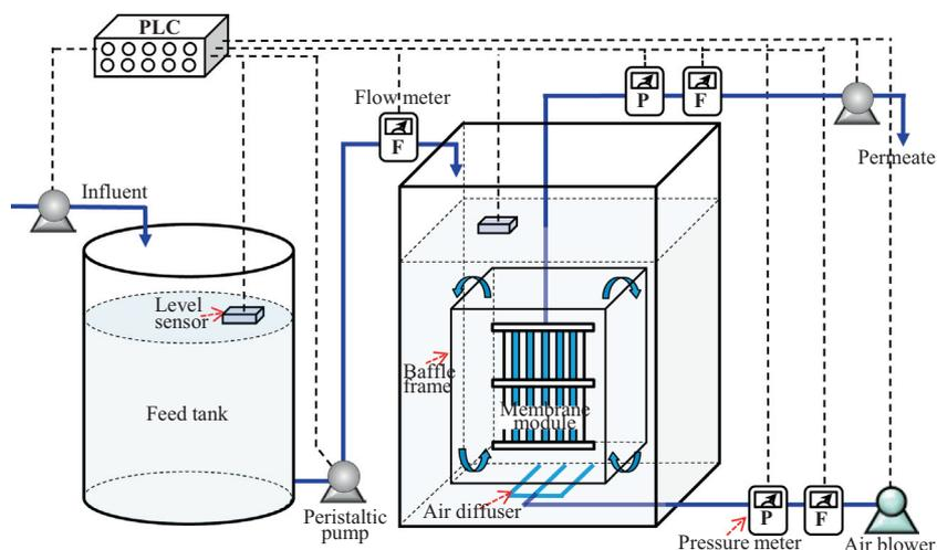
Fig. 1. Schematic design of the bench scale SMBR.
