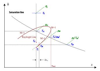
Fig. 1. The Mollier diagram for homogeneous nucleating in a vapor.
