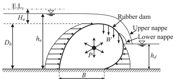
Fig. 1. Geometric and hydraulic features of a rubber dam.
