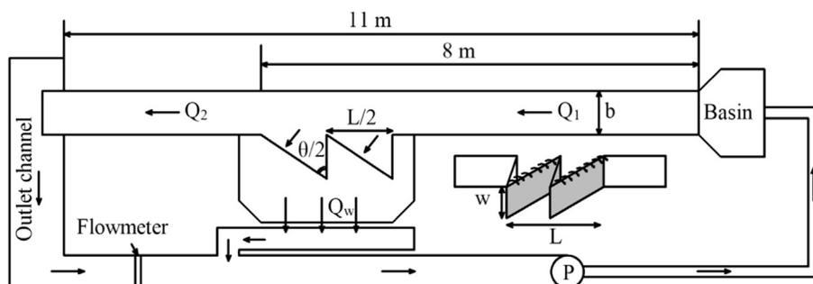
**Fig. 1.** Plan view of a modified oblique weir and the parameters used [21].
