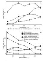
Effect of temperature on product yields of (A) gas, heavy oil, volatile organic compounds, and bio-oil; (B) solid residue, acid-soluble solid residue, acid-insoluble solid residue, water-soluble organics, ethanol-insoluble organics, and ethanol-soluble organics (conditions: reaction time of 0 min, 10 g of cornstalk, 100 ml of water).
