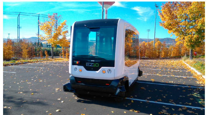
Fig. 1. EZ10, the bi-steerable vehicle used to evaluate our proposal
