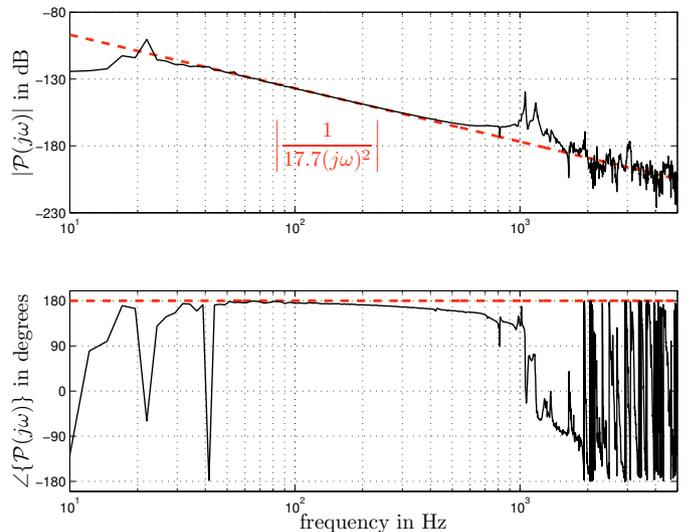
Fig. 3. Bode diagram of the measured frequency response data of a short-stroke wafer stage; 0dB = 1Nm<sup>-1</sup>.
