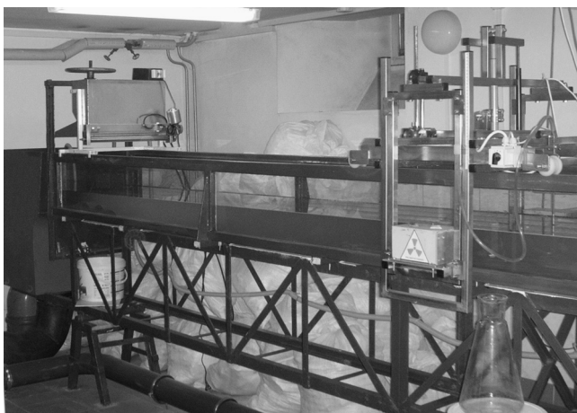
Fig. 2. The general view of the research installation with the radioisotope absorption set installed on the measuring trolley.
