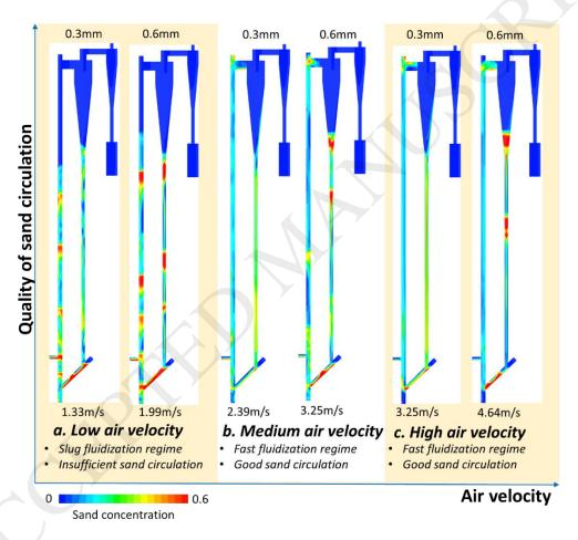
Contour snapshot of sand (0.3 mm and 0.6 mm) concentration (volume fraction) under different air velocity at steady conditions. Flow patterns of solids (silica sand) were obtained by linking the quality of solids recirculation with the air velocity and solids particle size.
