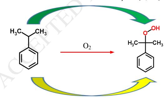
Conversion is 45.9% in 9 hours with Ionin liquid of  $[C_4 mim]OH$
