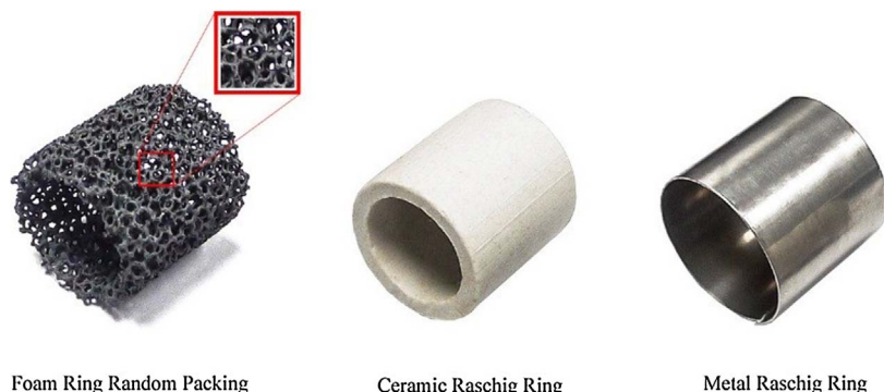
Fig. 1. Three kinds of ring packing used in the experiments.
