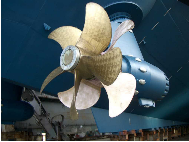
Fig. 2. Double pusher propeller aggregate of the ferry vessel “Schleswig-Holstein”, photo Scandlines archive
