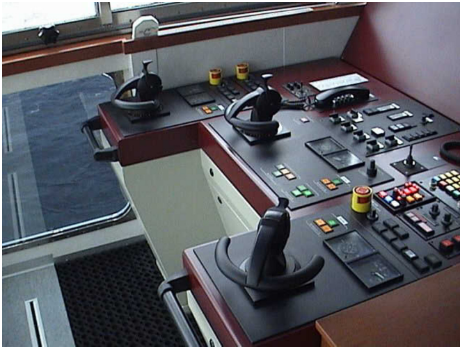
Fig. 3. Port wing control platform of the m/v “Arkona”, photo H. Korte
