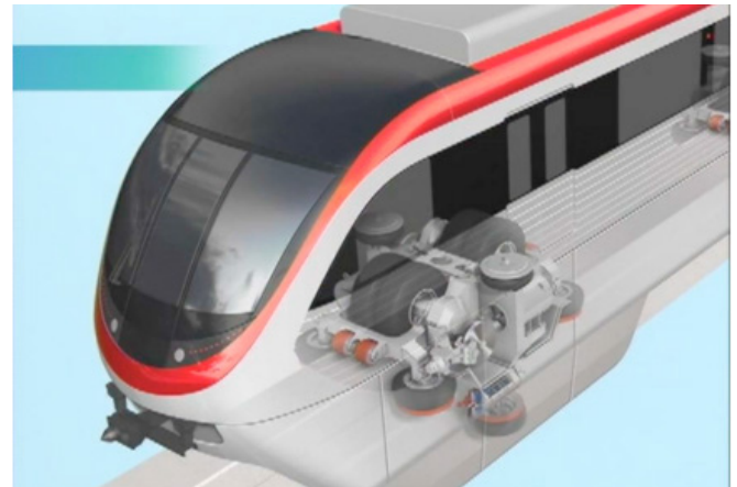
Fig. 1. The straddle type monorail of Hitachi (Hitachi Pres., 2013).
