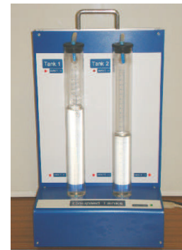
Fig. 1. Coupled tanks laboratory system
