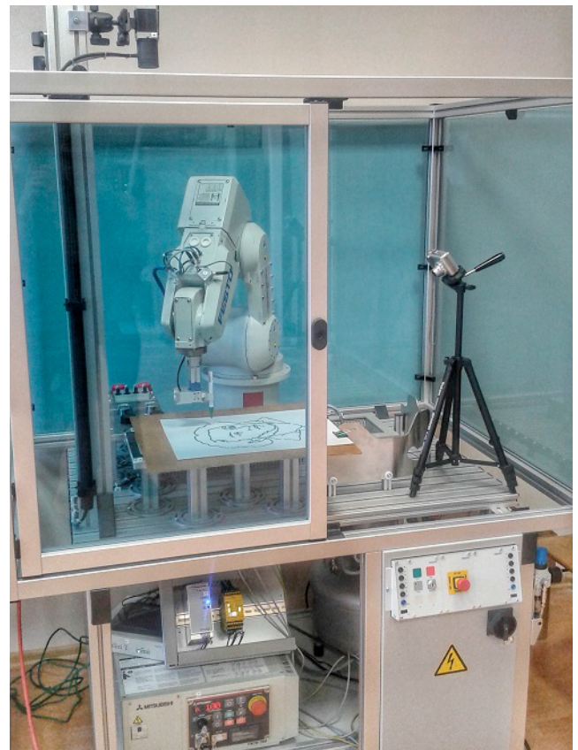
Fig. 2. The Festo Robot Vision Cell equipped with the robot Mitsubishi MELFA RV-3SDB
