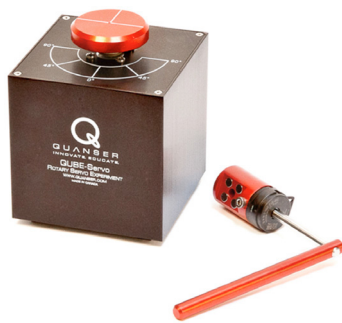
Fig. 1. Quanser© Qube TM -Servo platform
