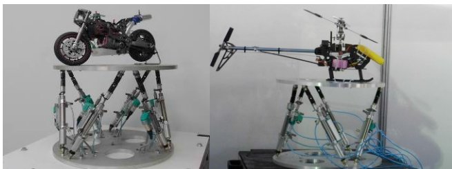
Figure 2. Stewart platform motion simulator with six degrees of freedom
