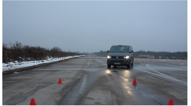
**Fig. 1.** *SC3-Bulli* experimental vehicle on test track during double lane change manoeuvre.
