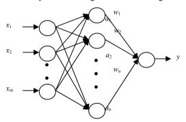
Note)  $x_m$ : input data,  $w_n$ : weights of between input and hidden layers,  $a_n$ : output of hidden layer, y: output
