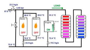
Fig. 1: Schematic diagram of a CHP
