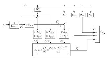
Fig. 1. The MATLAB/ Simulink realization of SOFC model.
