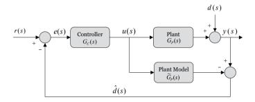
Fig. 2. Block diagram of internal model control (IMC).
