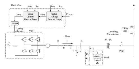
Fig. 1. Schematic diagram of the study system.
