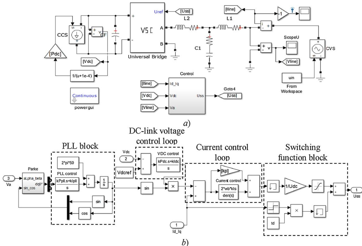
Fig. 1. Simulink-based model of a single-phase PV inverter (a) and schematic of respective control system (b).
