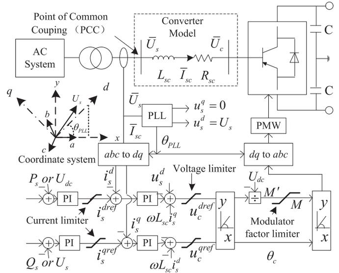
Fig. 2. A single-line diagram of a converter and its control systems.
