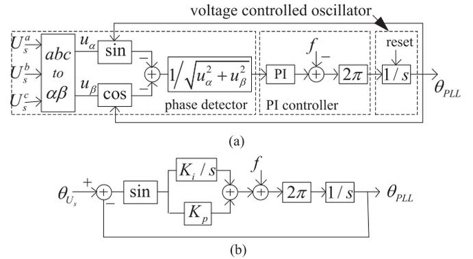
Fig. 3. Control block diagram of the PLL. (a) Detail PLL topology for EMTPs (b) simplified PLL topology for TSPs.
