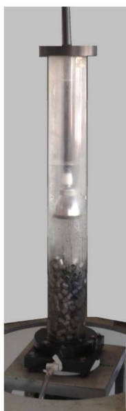
Fig. 3. Scheme (a) and picture (b) of the experimental random packed column.
