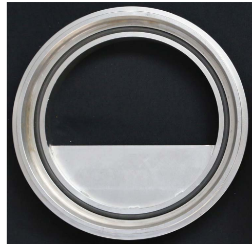
Fig. 1. The segmental orifice plate. The lower third of the pipe's cross section is covered by a horizontal restriction.
