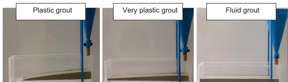
Fig. 3. Profiles flow depending on the grout viscosity.
