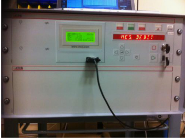
Fig. 1. A front view of the micro-flow transfer standard ( \mu\text{FTS} ).
