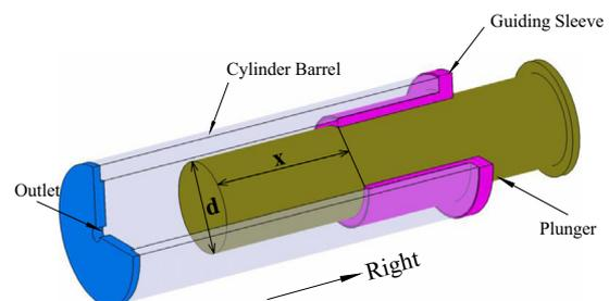
Fig. 2. Structure diagram of the metering cylinder.
