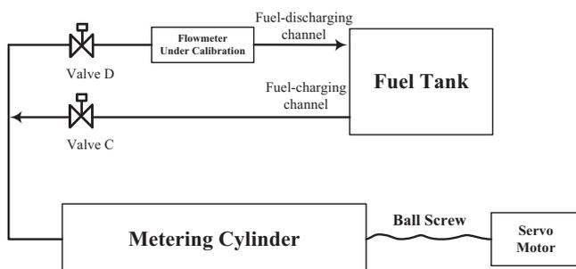
Fig. 1. Schematic of the calibration system.
