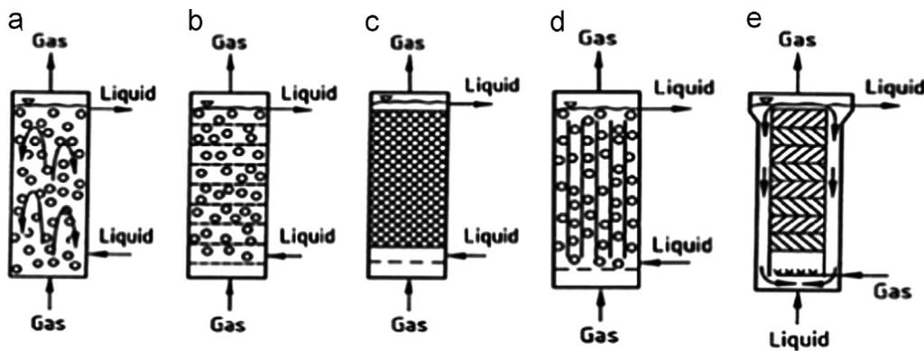
Fig. 1. Types of bubble column reactors [8].
