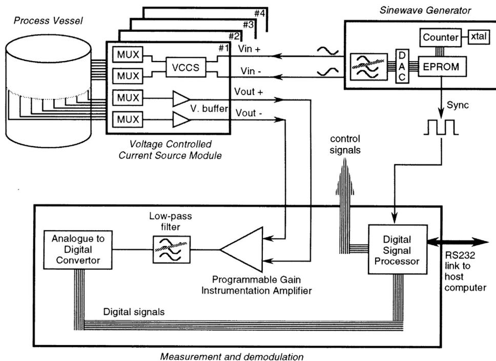
Fig. 2. An electrical resistance tomography data acquisition system [17].
