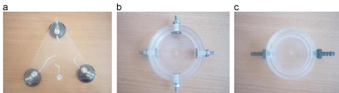
Fig. 1. Three parts of the spectroscopy equipment design: (a) base, (b) vessel and (c) gas chamber cap.
