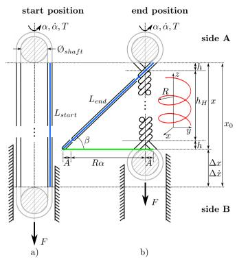
Fig. 2. Model of string transmission: (a) shows the string in its original condition ( $\alpha=0,\dot{\alpha}=0$  and T=0). (b) is for  $\alpha>0$ .
