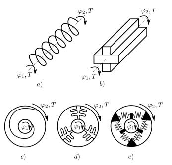
Fig. 1. Possible spring types in SEAs: a) classic torsion spring, b) cantilever spring, c) and d) monolithic structured spring element, e) circular structure with classic springs.
