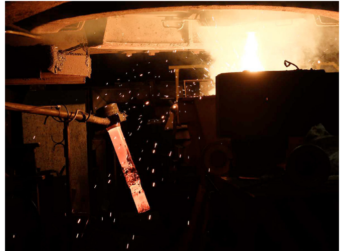
Fig. 2. Molten metal reacting to atmospheric oxygen (right) when the shroud pipe (left) is removed. (Courtesy of ŽP Research and Development Centre.)
