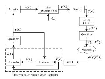
Fig. 1. Event-triggered networked control system structure.
