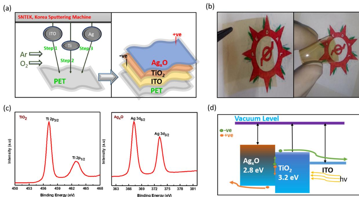
Fig. 1. (a) Fabrication steps and schematic diagram, (b) device photographs, (c) XPS spectra of Ti and Ag and (d) Energy band diagram.
