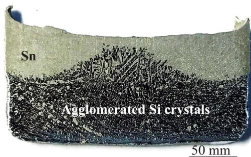
Fig. 2. Cross-section of Sn–60 at% Si alloy after the solidification refining process with electromagnetic separation.
