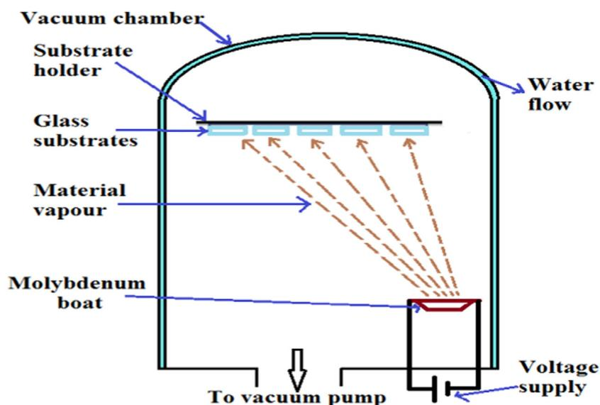
Fig. 1. Arrangement of glass substrates with respect to the source in the vacuum chamber.
