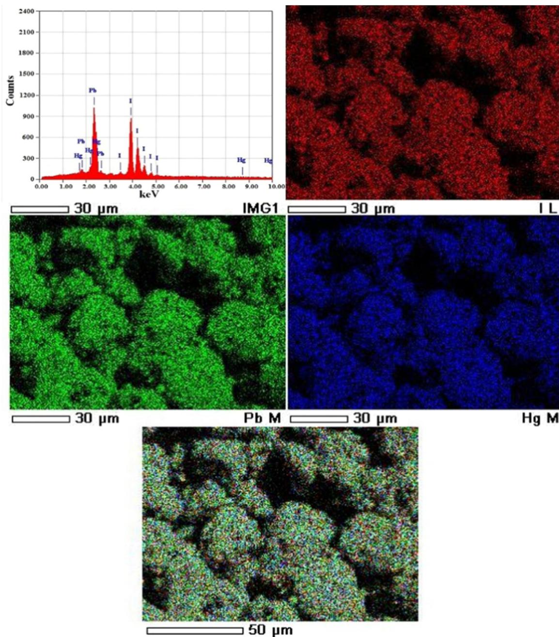
Fig. 1. EDX and SEM mapping images of 2.5% Hg doped  $\text{PbI}_2$  nanostructures.
