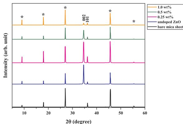
Fig. 2. XRD patterns for bare mica sheet, ZnO and different Al doped ZnO (AZO).
