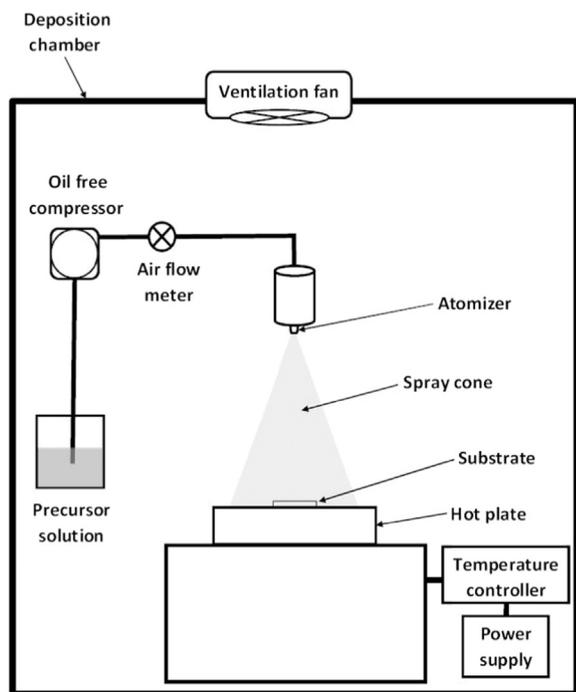
Fig. 1. The schematic diagram of the spray pyrolysis system.
