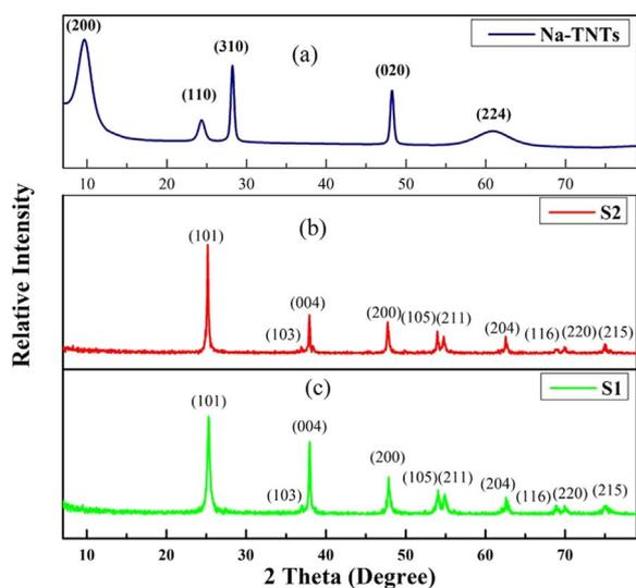
Fig. 2. (a-c) XRD patterns of Na-TNTs, S2 and S1, respectively.
