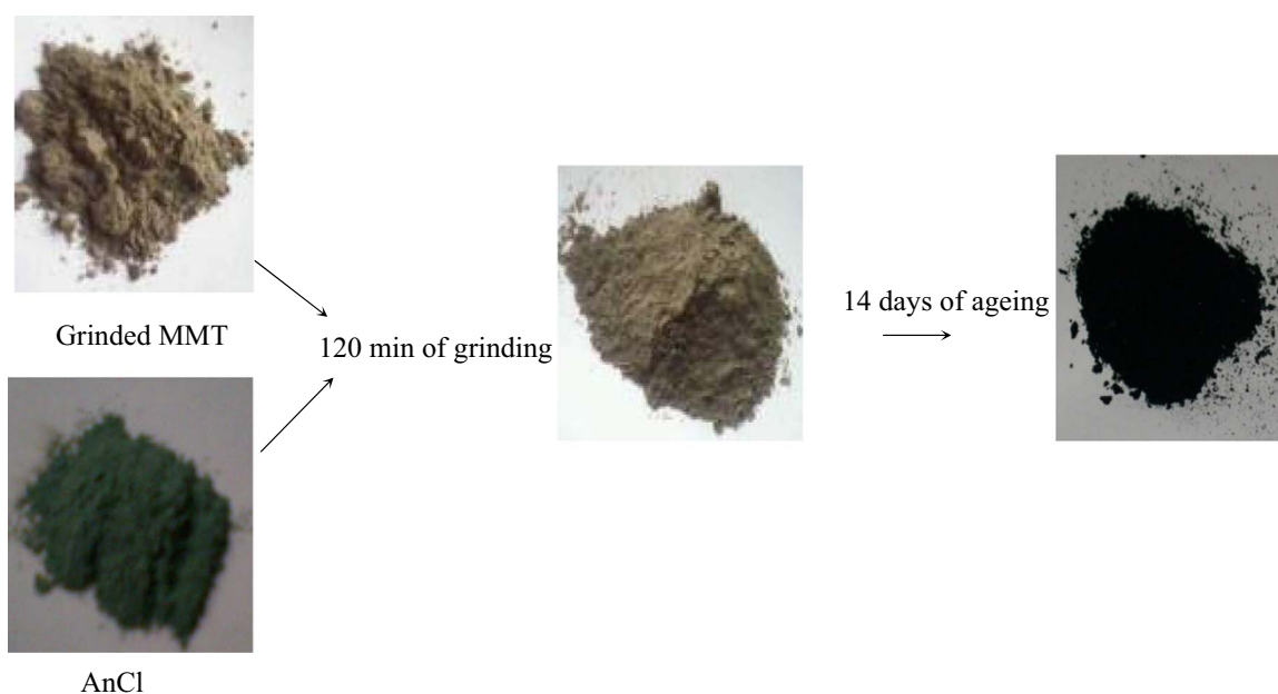
Fig. 1. Evolution of color with grinding and ageing of the grinded mixture of aniline chloride with grinded MMT (The molar ratio of (structural iron / \text{AnCl} )=0.12). (For interpretation of the references to color in this figure legend, the reader is referred to the web version of this article.)
