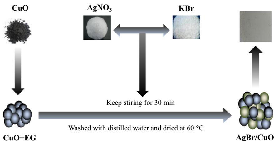
Scheme 1. Preparing procedure of AgBr/CuO hybrid photocatalysts.
