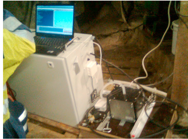
Fig. 1. The NMR device modified for online measurements in an industrial condition.
