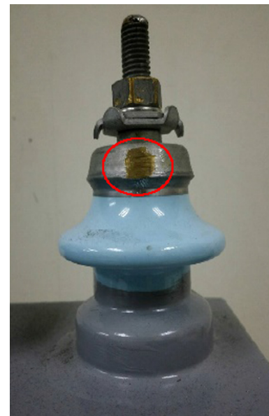
Fig. 2. Metal sleeve wear.
